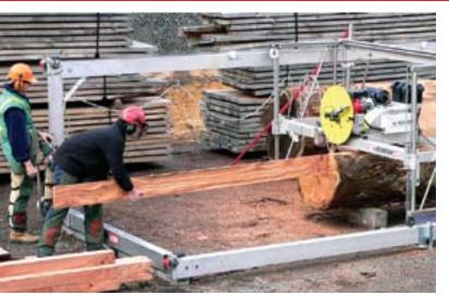
The Automated Swingblade Mill (ASM) delivers fast and consistent production with little operator fatigue, while maintaining a high level of portability.
